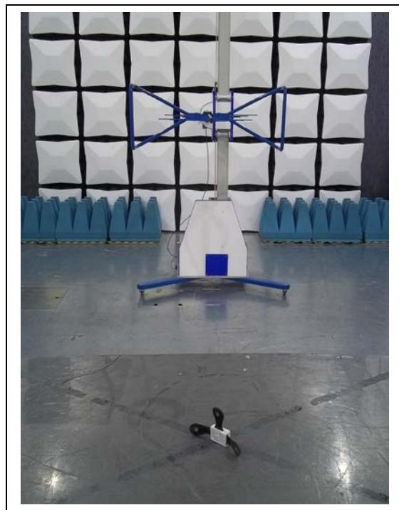
**Radiated Spurious Emissions, 1 GHz to 18 GHz**
