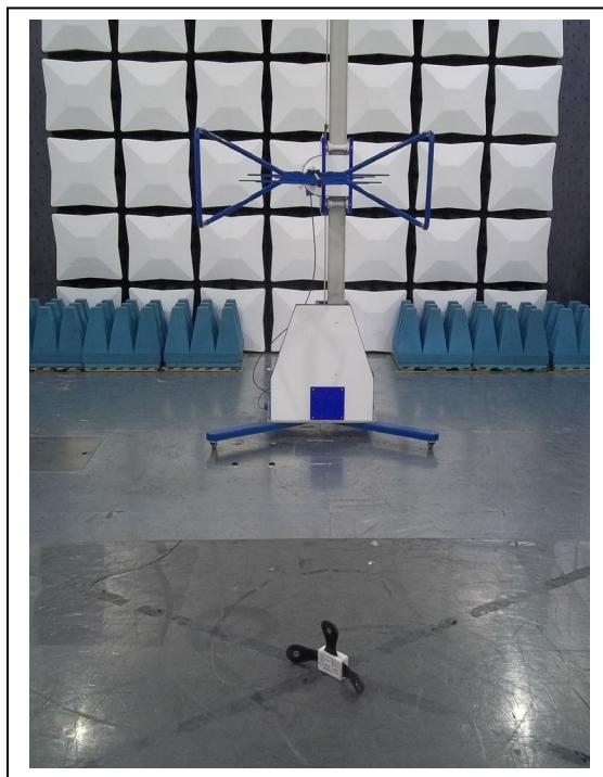
**Radiated Spurious Emissions, 1 GHz to 18 GHz**
