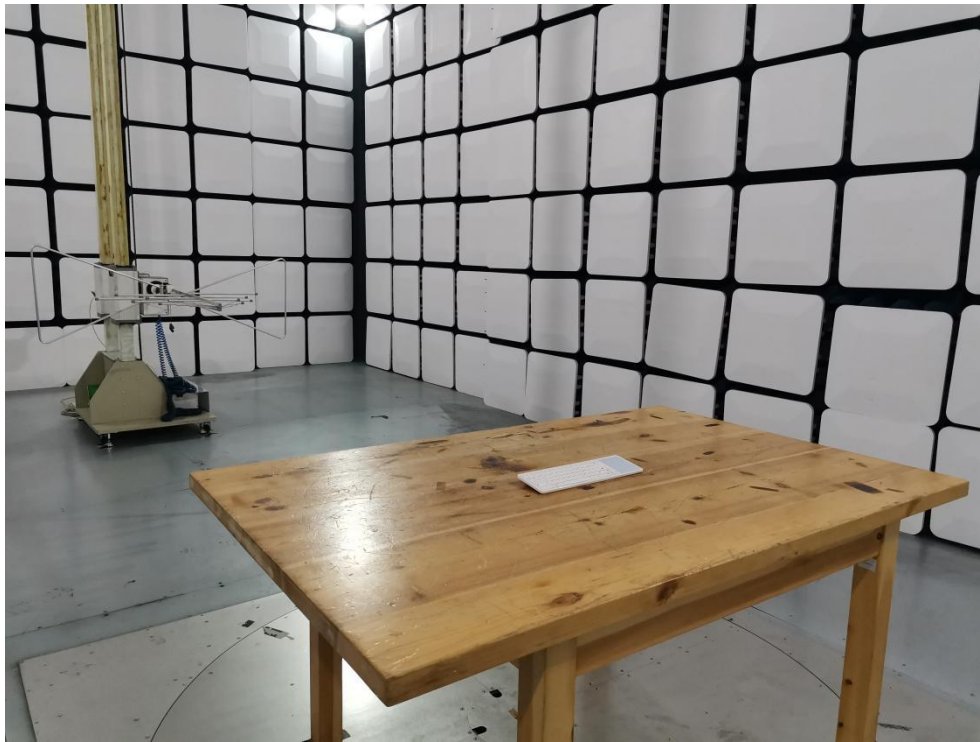
FCC ID: 2AQS3-CK118G Photo of Radiation Emission Test
