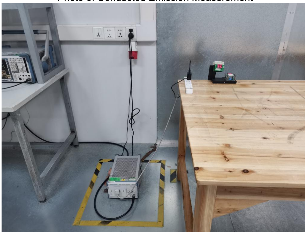
FCC ID: 2AQRPTJC157WC Photo of Conducted Emission Measurement
