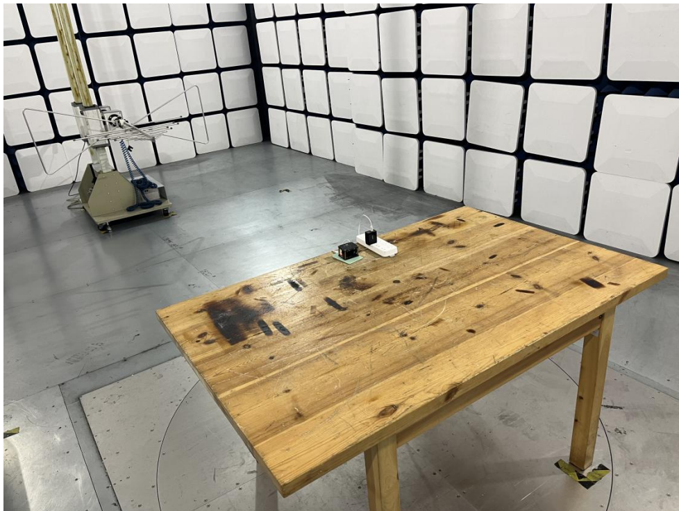
Photo of Radiation Emission Test
