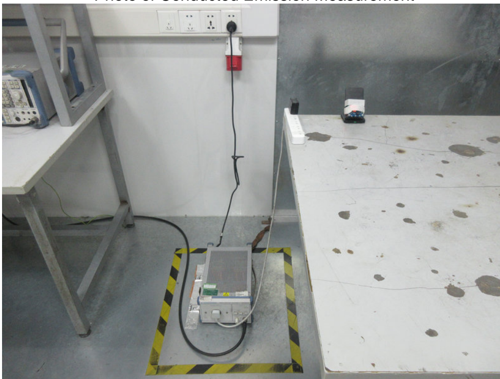
FCC ID: 2AQRPTJC05610W Photo of Conducted Emission Measurement
