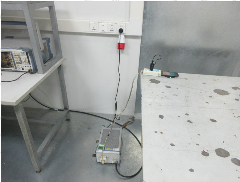
Photo of Conducted Emission Measurement
