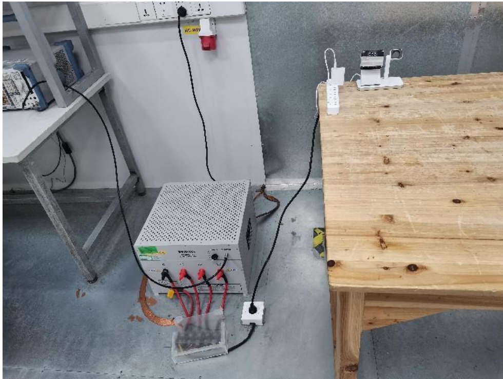
FCC ID: 2AQRP-C-093 Photo of Conducted Emission Measurement
