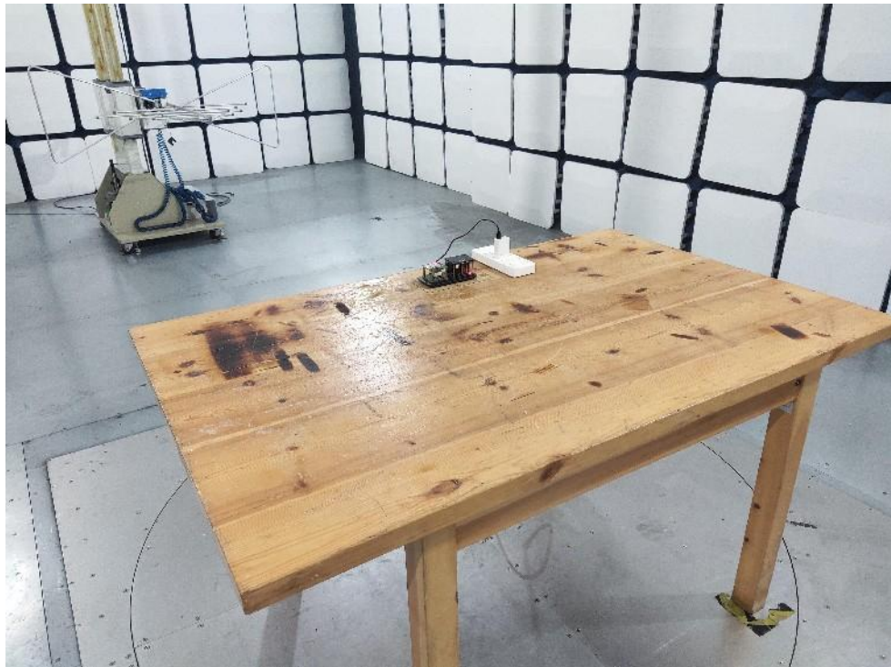
Photo of Radiation Emission Test
