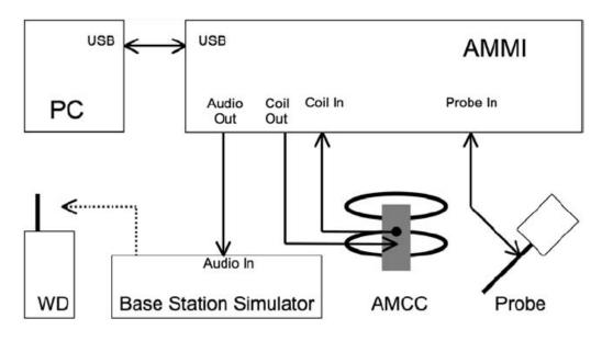
Figure 5.2 T-Coil setup with HAC Test Arch and AMCC
