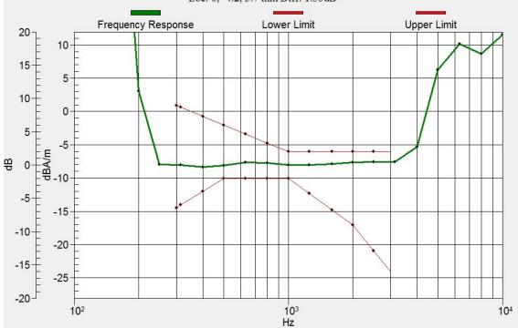
Figure C.9 Frequency Response of LTE B12
