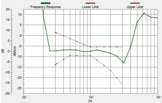
Figure C.6 Frequency Response of LTE B2
