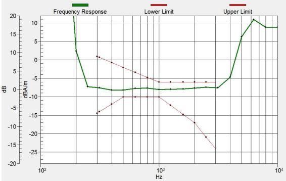
Figure C.14 Frequency Response of LTE B71
