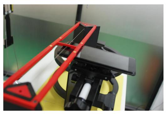
Picture 2: EUT Positioning for RF/T-coil
