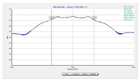
Fig.20. 6dB Bandwidth: GFSK, 2402 MHz
