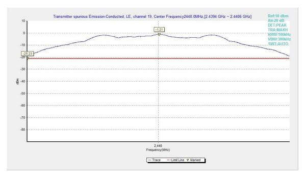
Fig.8. Transmitter Spurious Emission -Conducted: GFSK, 2440MHz
