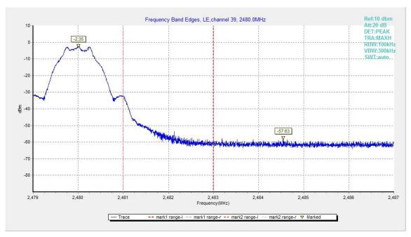
Fig.2. Frequency Band Edges: GFSK, 2480 MHz, Hopping Off
