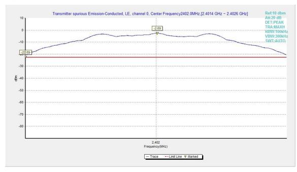
Fig.3. Transmitter Spurious Emission -Conducted: GFSK,2402MHz
