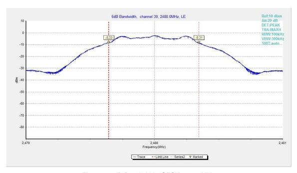
Fig.22. 6dB Bandwidth: GFSK, 2480 MHz
