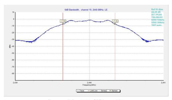
Fig.21. 6dB Bandwidth: GFSK, 2440 MHz
