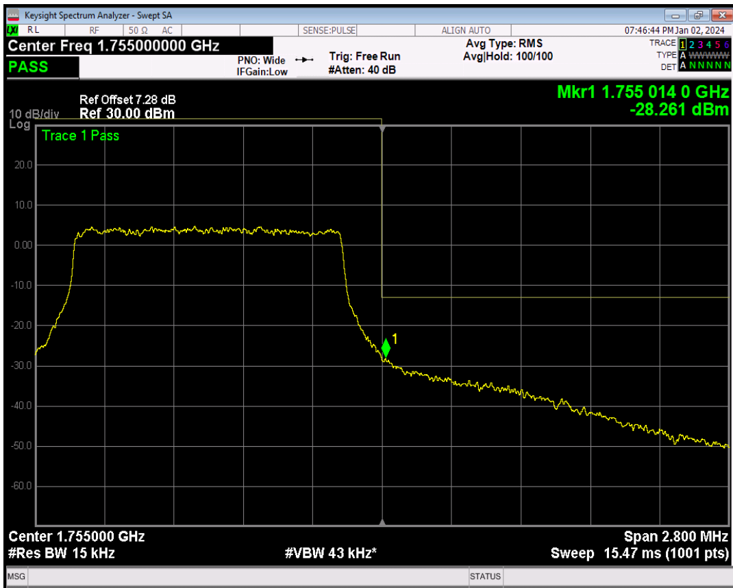
Band4 QPSK BW=10MHz Channel=20350 RB Size=1 Position=#Max
