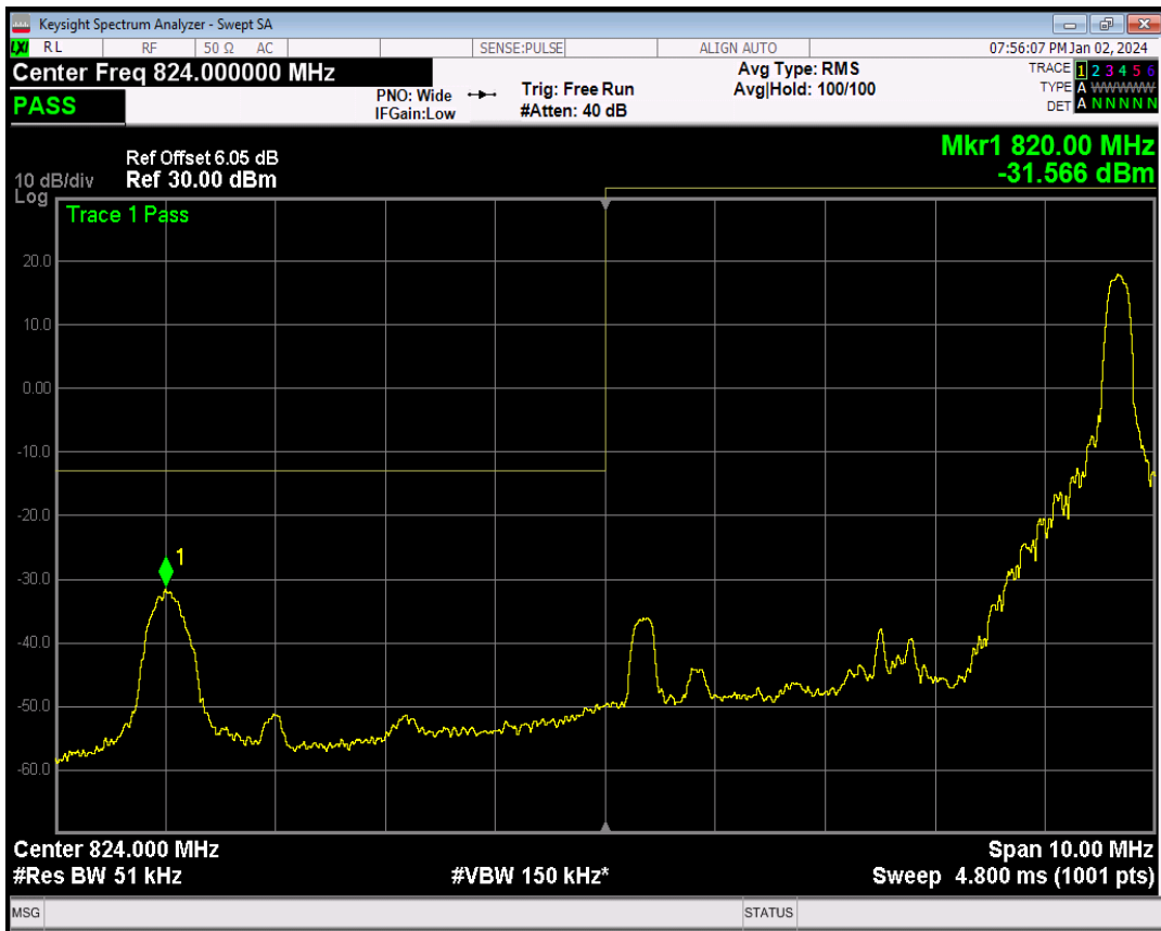
Band5 QPSK BW=3MHz Channel=20635 RB Size=15 Position=#0
