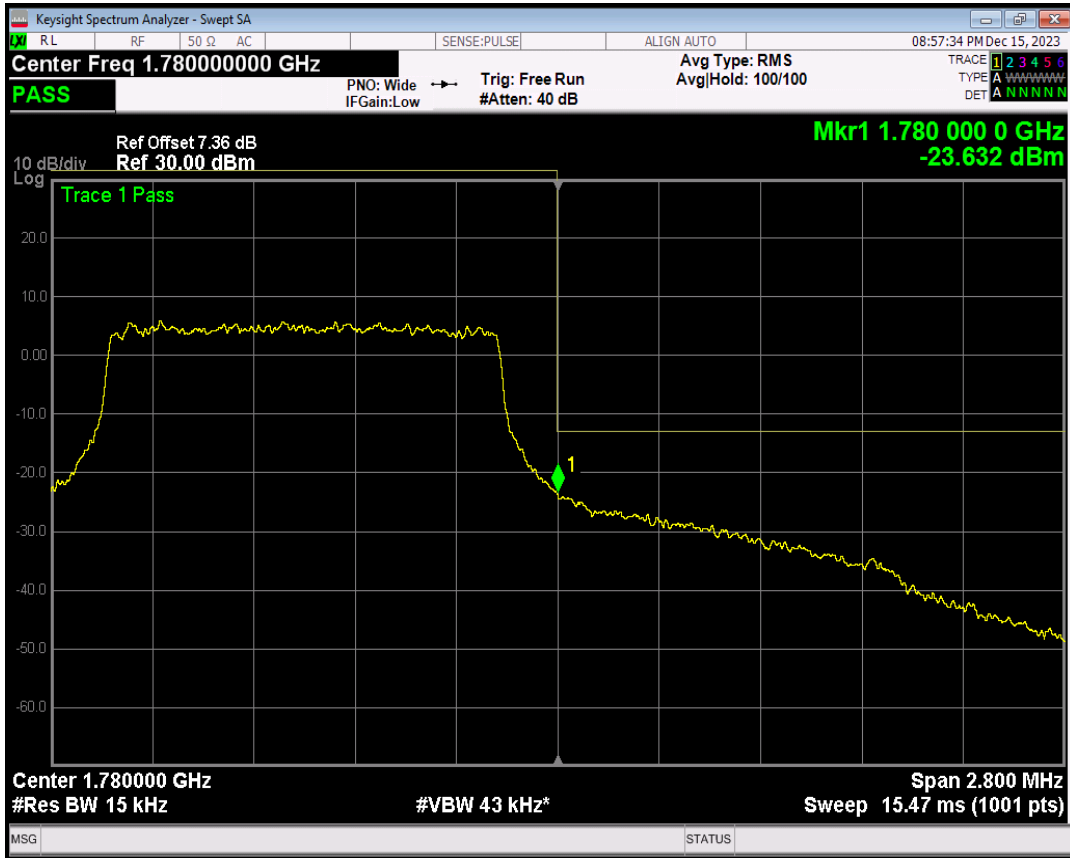
Band66 16QAM BW=1.4MHz Channel=132665 RB Size=1 Position=#0
