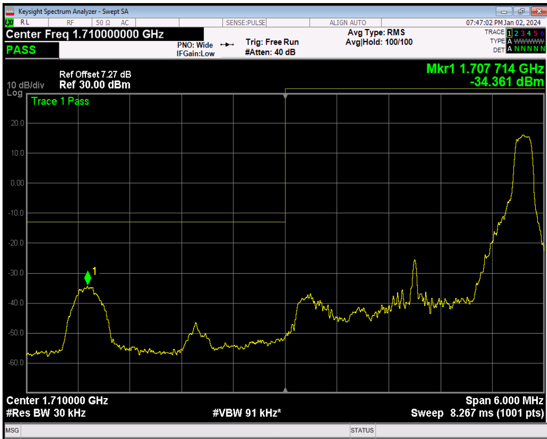
Band4 QPSK BW=3MHz Channel=19965 RB Size=15 Position=#0
