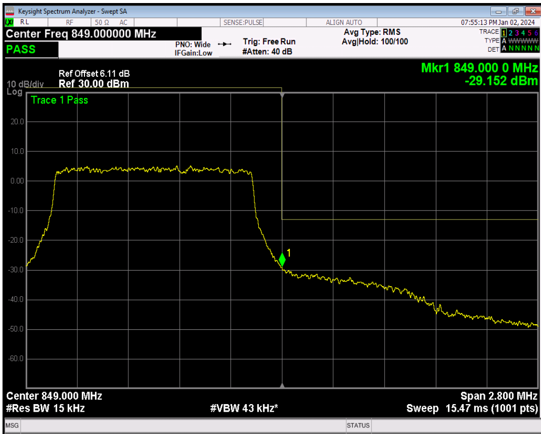
Band5 QPSK BW=10MHz Channel=20450 RB Size=1 Position=#0
