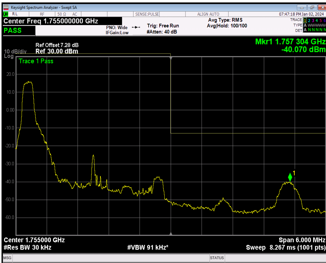
Band4 QPSK BW=3MHz Channel=20385 RB Size=1 Position=#Max
