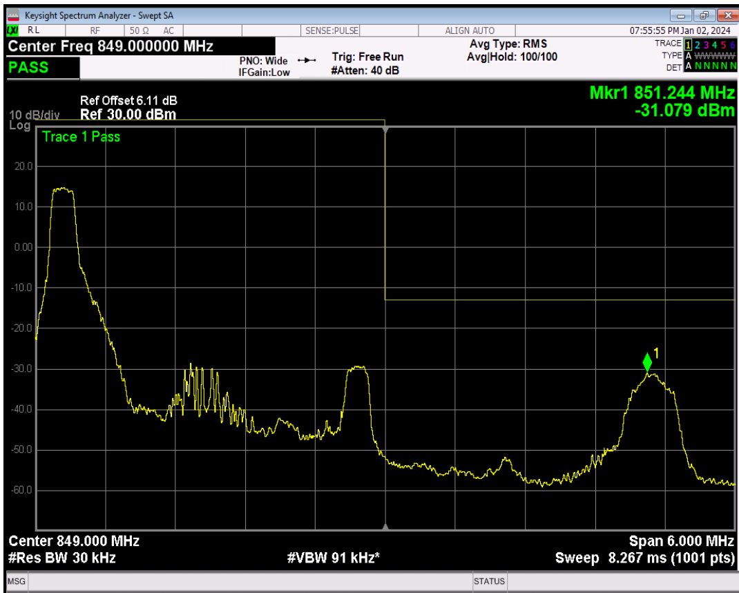
Band5 16QAM BW=3MHz Channel=20635 RB Size=1 Position=#Max
