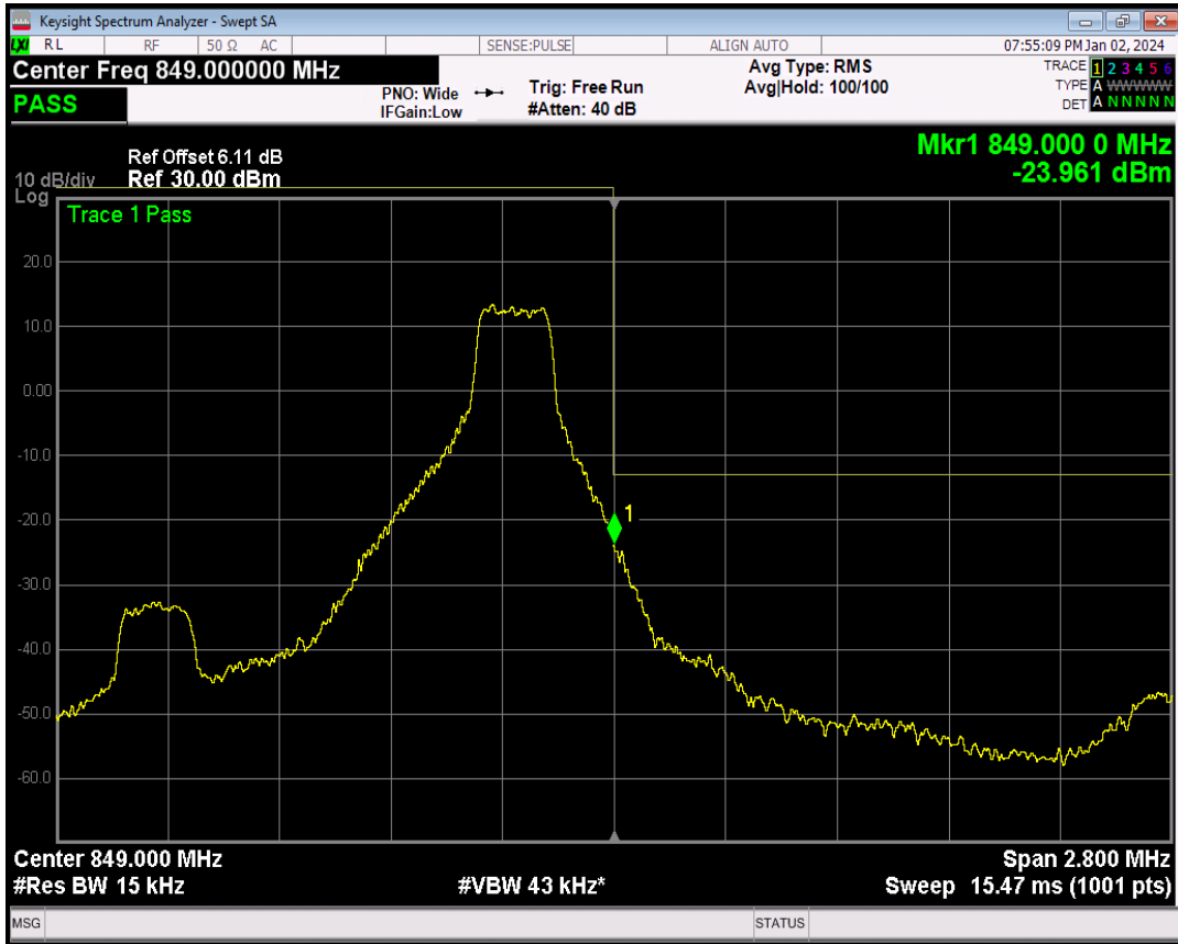
Band5 QPSK BW=10MHz Channel=20600 RB Size=1 Position=#Max
