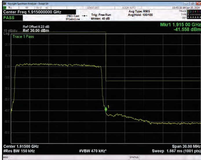
Band25 QPSK BW=20MHz Channel=26140 RB Size=1 Position=#0 Normal
