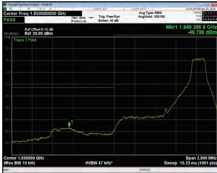
Band25 QPSK BW=1.4MHz Channel=26047 RB Size=6 Position=#0 Normal
