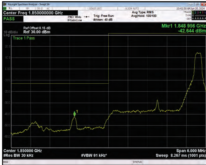
Band25 QPSK BW=3MHz Channel=26055 RB Size=15 Position=#0 Normal
