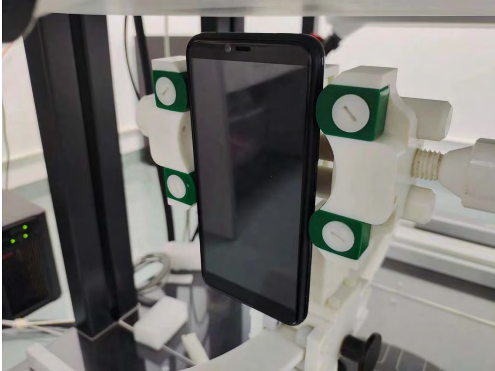
Body Top side (separation distance is 10mm)
