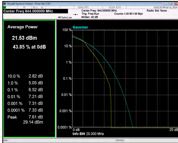
Band5 16QAM BW=3MHz Channel=20415 RB Size=1 Position=#0
