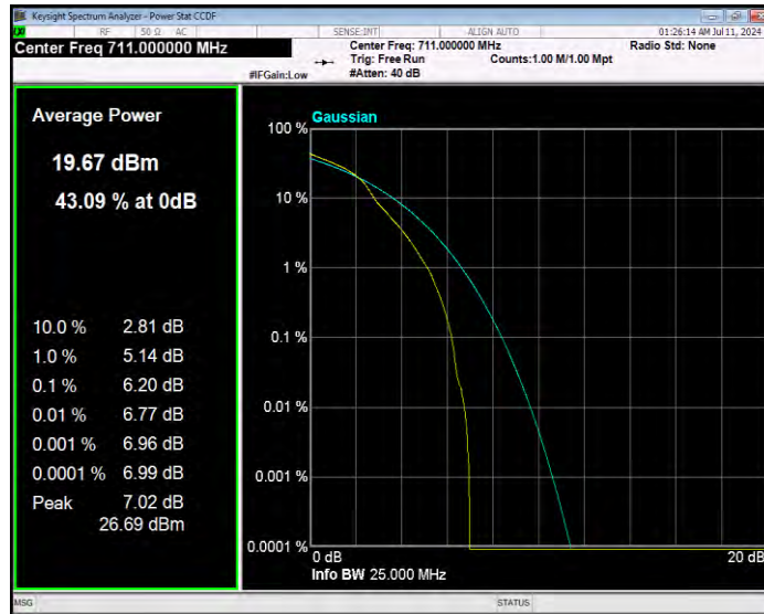
Band17 16QAM BW=5MHz Channel=23755 RB Size=1 Position=#0
