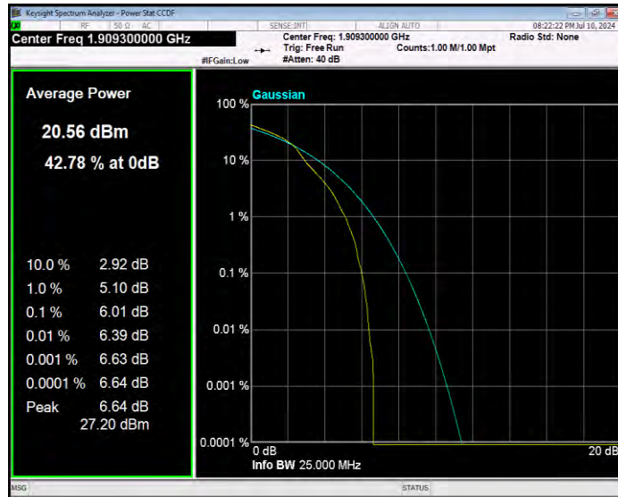
Band2 16QAM BW=10MHz Channel=18650 RB Size=1 Position=#0
