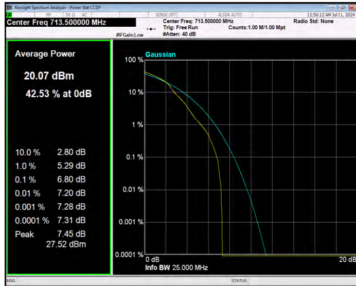
Band12 QPSK BW=1.4MHz Channel=23017 RB Size=1 Position=#0
