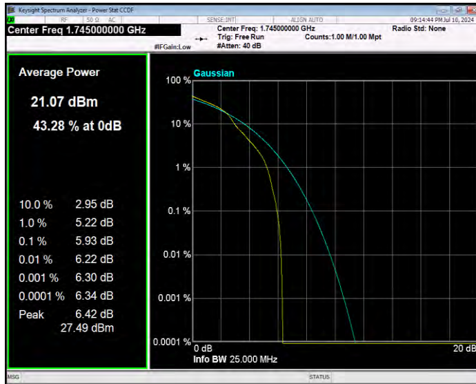
Band4 16QAM BW=3MHz Channel=19965 RB Size=1 Position=#0
