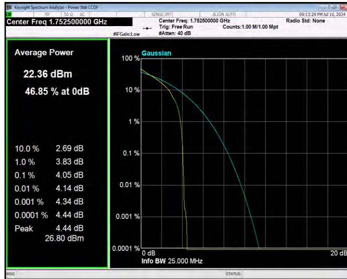
Band5 16QAM BW=1.4MHz Channel=20407 RB Size=1 Position=#0
