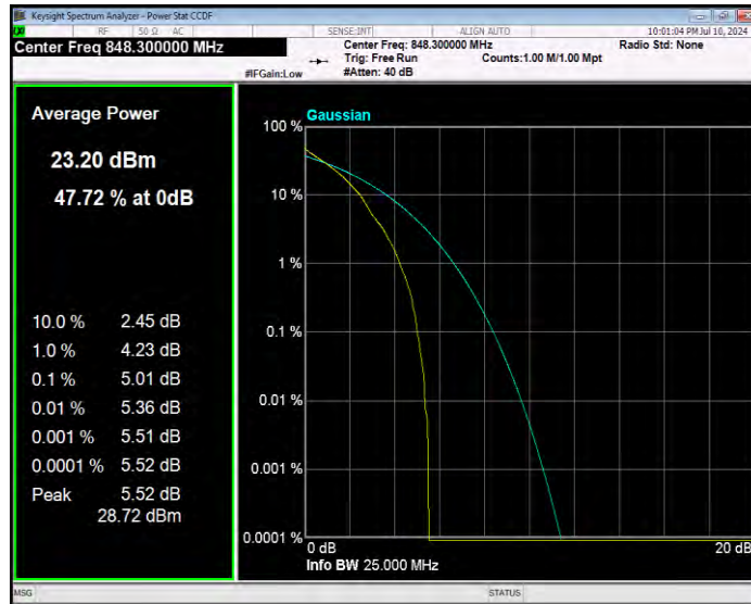
Band5 QPSK BW=10MHz Channel=20450 RB Size=1 Position=#0
