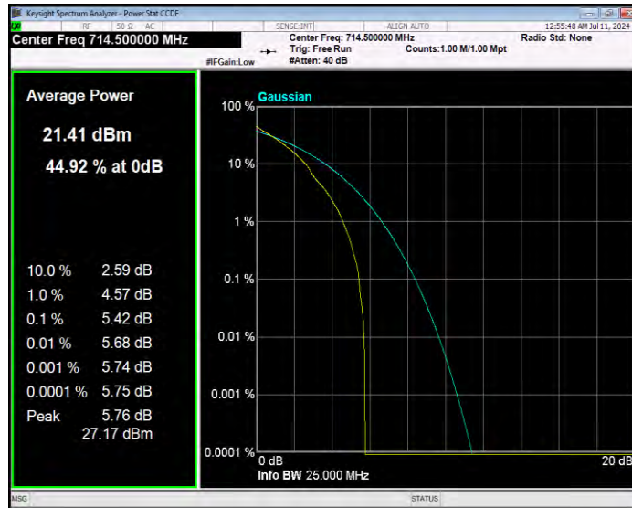
Band12 QPSK BW=5MHz Channel=23035 RB Size=1 Position=#0
