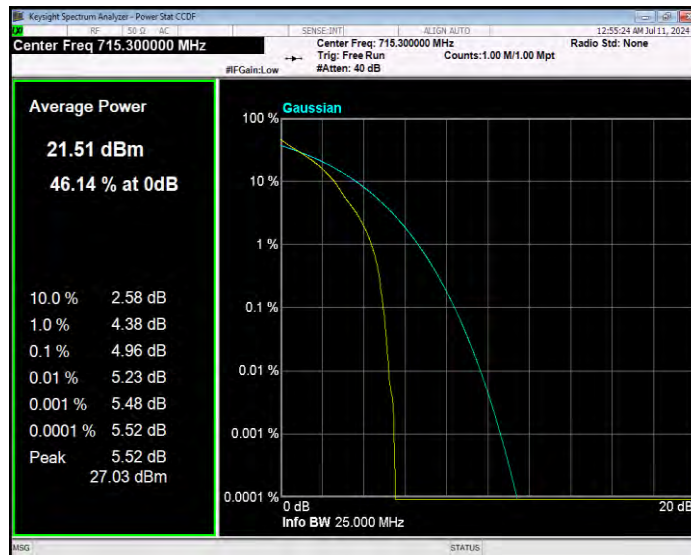
Band12 QPSK BW=10MHz Channel=23060 RB Size=1 Position=#0
