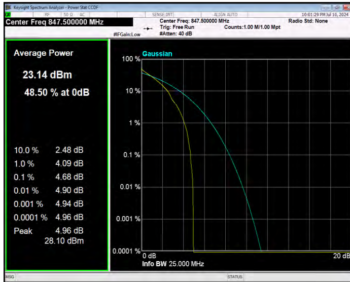
Band5 QPSK BW=5MHz Channel=20425 RB Size=1 Position=#0
