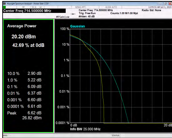
Band12 16QAM BW=5MHz Channel=23035 RB Size=1 Position=#0
