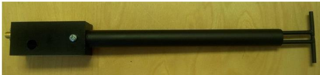
Figure 1 – MVG COMOSAR Validation Dipole
