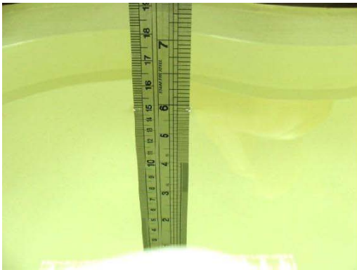
Fig 7.1 Photo of Liquid Height for Head SAR
