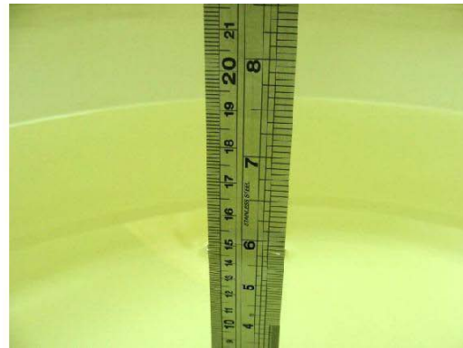
Fig 7.2 Photo of Liquid Height for Body SAR
