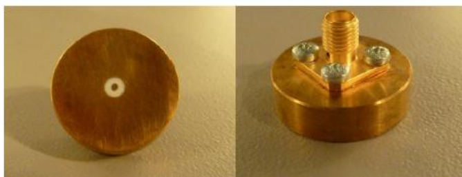
Figure 1 – MVG LIMESAR Dielectric Probe
