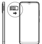
NOTE: Some applications may require a microSD card to work normally or may store certain data on it. Therefore, it is recommended that you keep a microSD card installed and not remove or replace it randomly.
