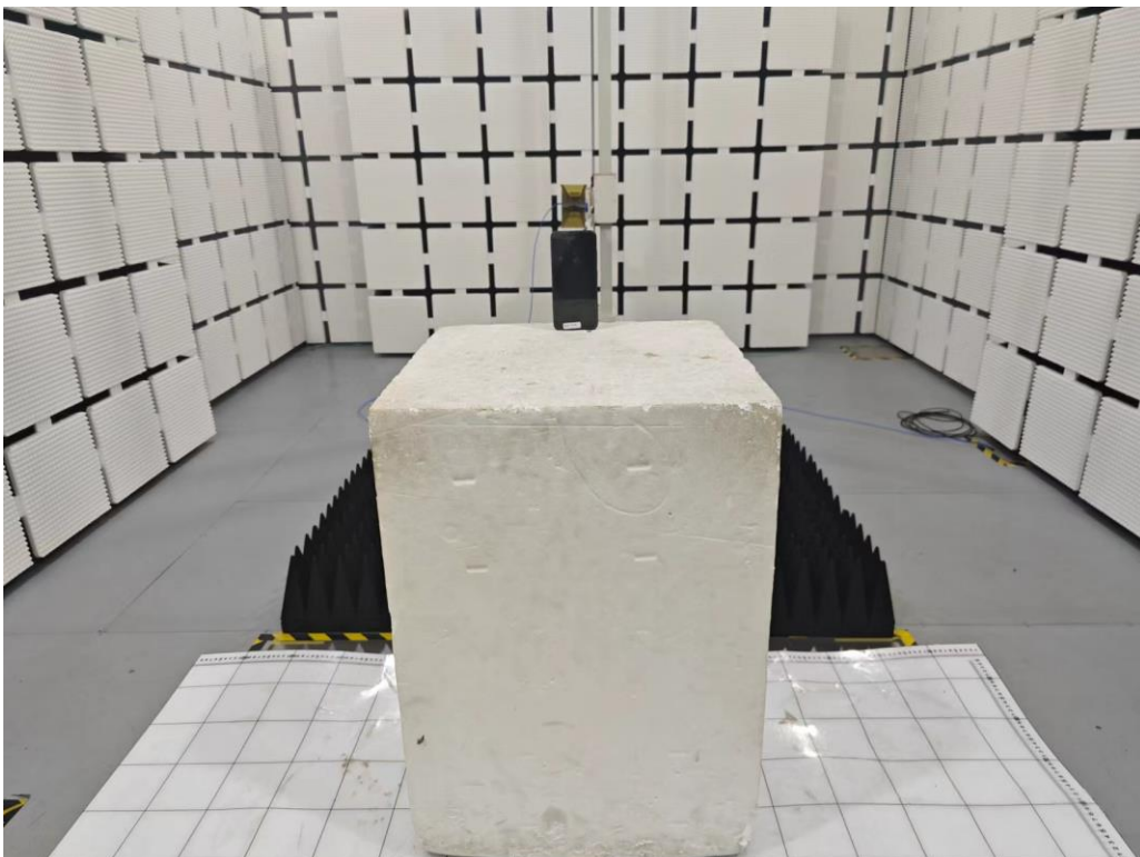
Set-up for Radiated Spurious Emission, Above 1GHz
