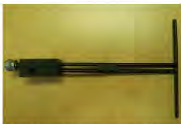
Figure 1 – MVG COMOSAR Validation Dipole
