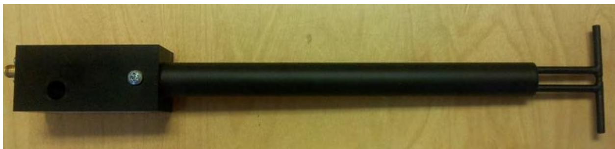
Figure 1 – MVG COMOSAR Validation Dipole
