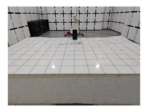
Set-up for Radiated Spurious Emission, Above 1GHz
