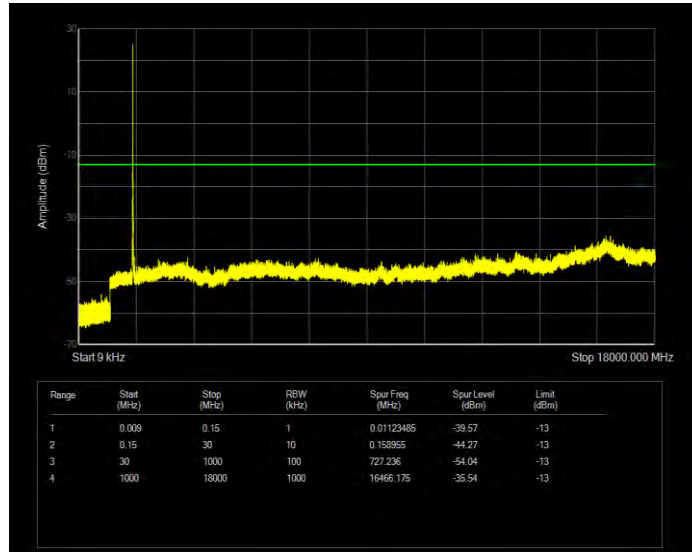
Band66 QPSK BW=3MHz Channel=131987 RB Size=15 Position=#0
