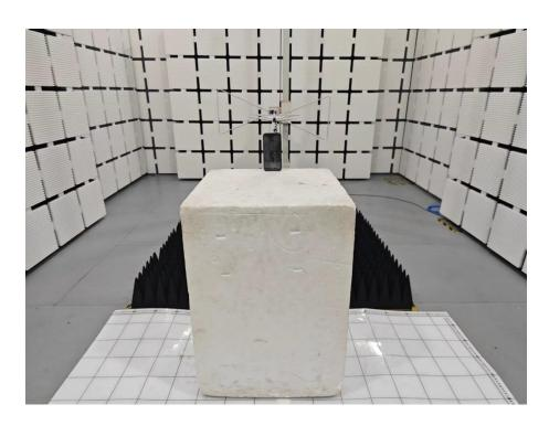
Set-up for Transmitter & Receiver Spurious Emissions, Above 1GHz
