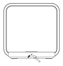
• Insert the adaptor head into the socket behind the lamp.
