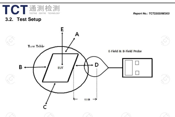
Note: Measurements should be made from all sides and the top of the primary/client pair, with the 15cm measured from the center of the probe(s) to the edge of the device.
