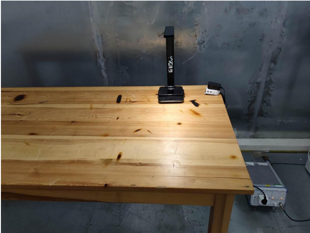
Conducted Emission-AC adapter charge mode
