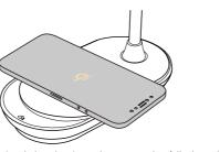
Notice: the light indicator is red when charging, and turn green when fully charged, if the red light is flashing, it means charging failure.
