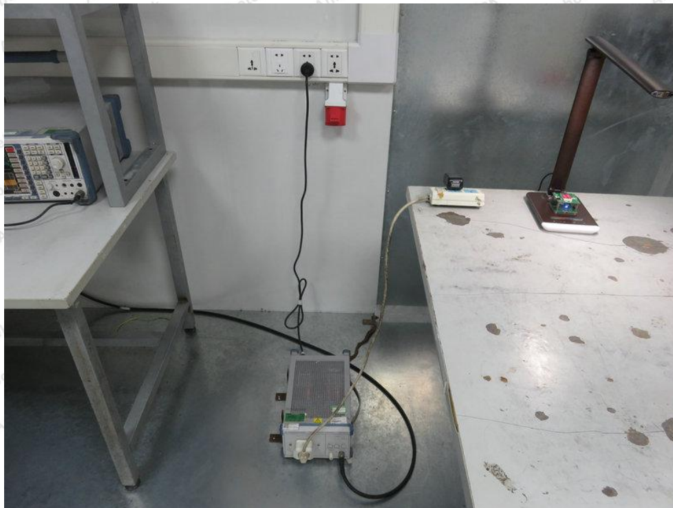
Photo of Conducted Emission Measurement
