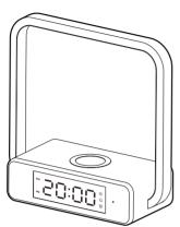
Plug in the power adapter, the display automatically turns on, the buzzer beeps twice, and the wireless charging indicator lights up red and green at the same time.
