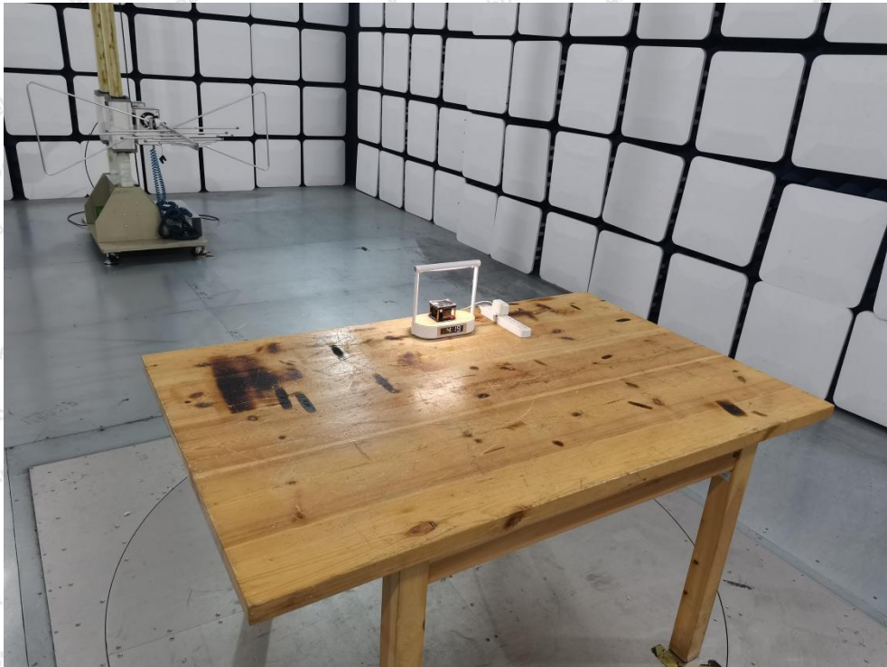
Photo of Radiation Emission Test
