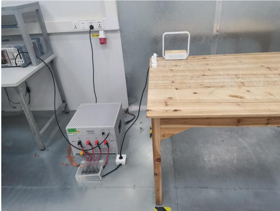
Photo of Conducted Emission Measurement
