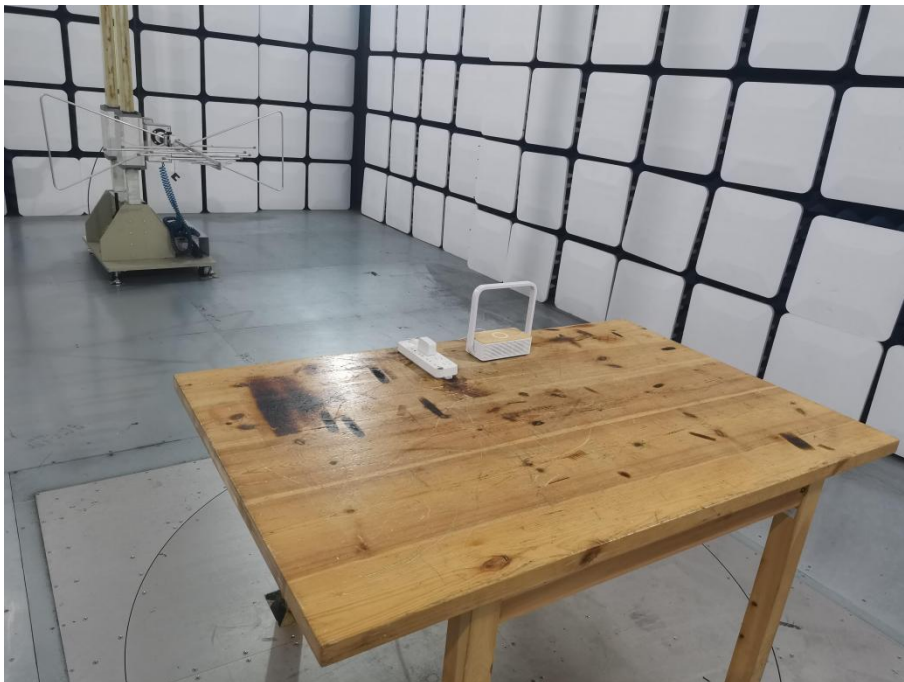
Photo of Radiation Emission Test
