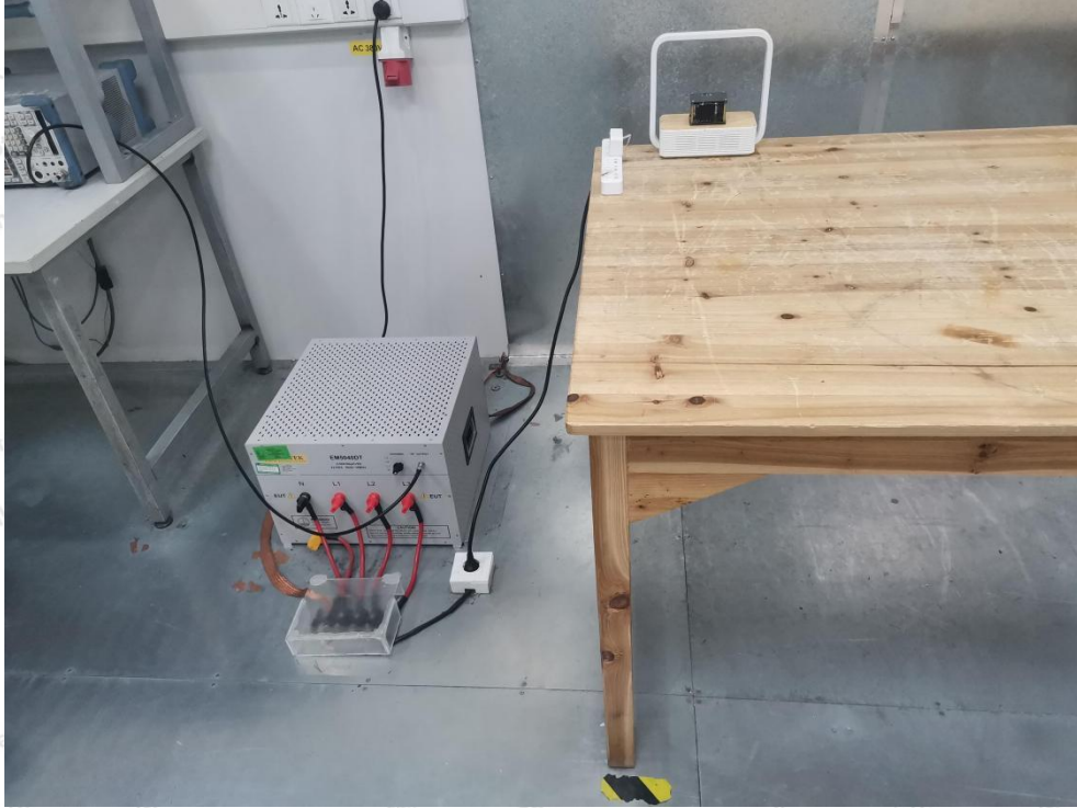
Photo of Conducted Emission Measurement
