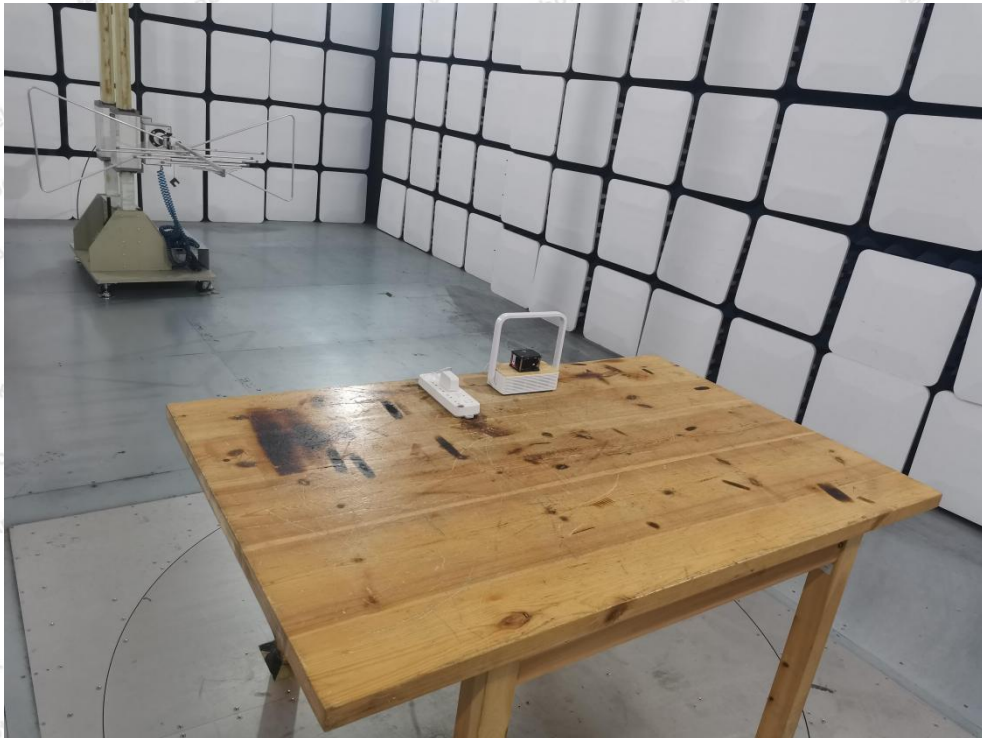
Photo of Radiation Emission Test
