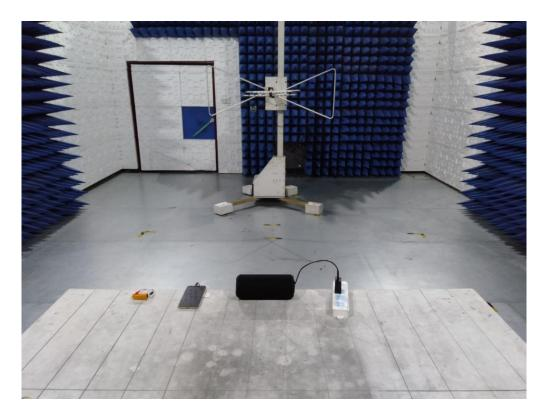
RADIATED EMISSION TEST SETUP ABOVE 1GHZ
