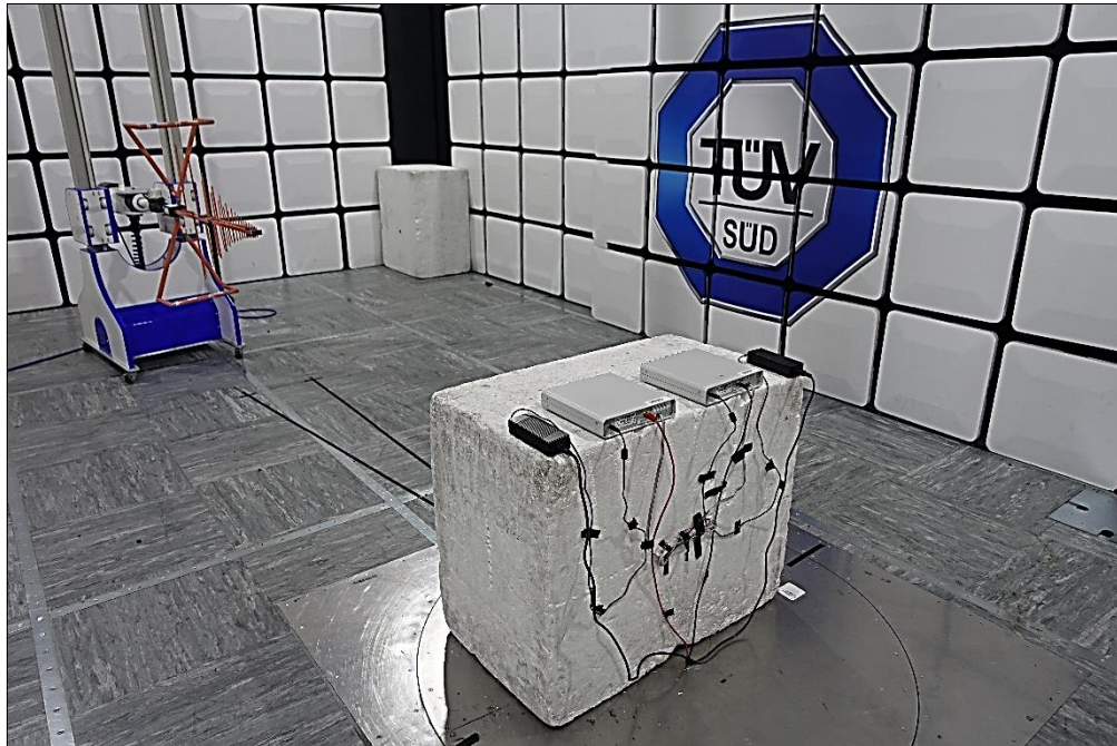
Figure 9 - Test Setup - 30 MHz to 1 GHz
