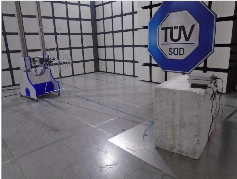
Figure 30 - Test Setup - 30 MHz to 1 GHz
