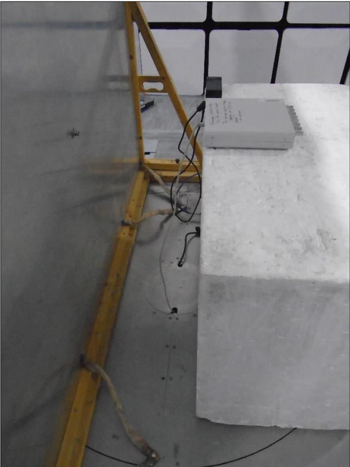
Figure 61 - AC Line Conducted Emissions
