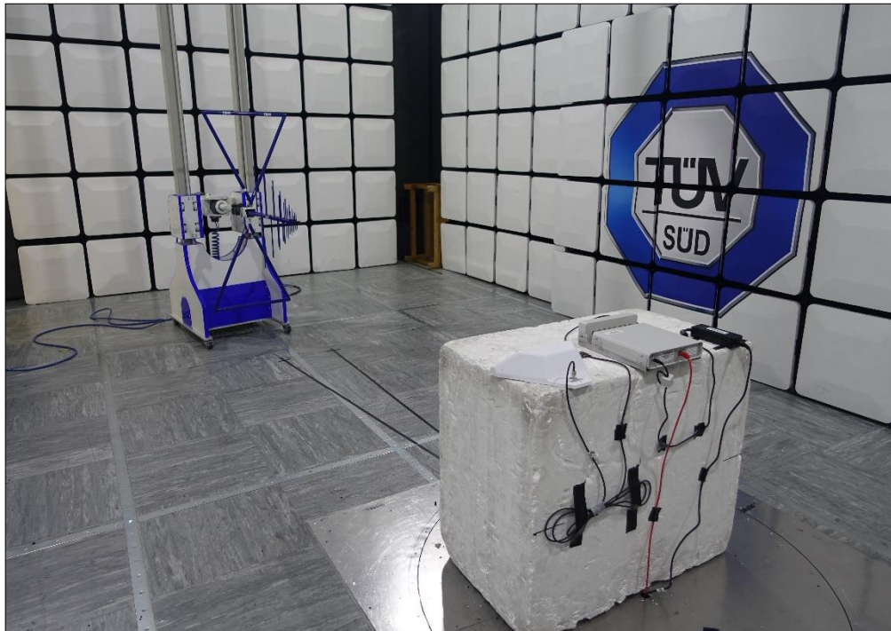
Figure 17 - Test Setup - 30 MHz to 1 GHz
