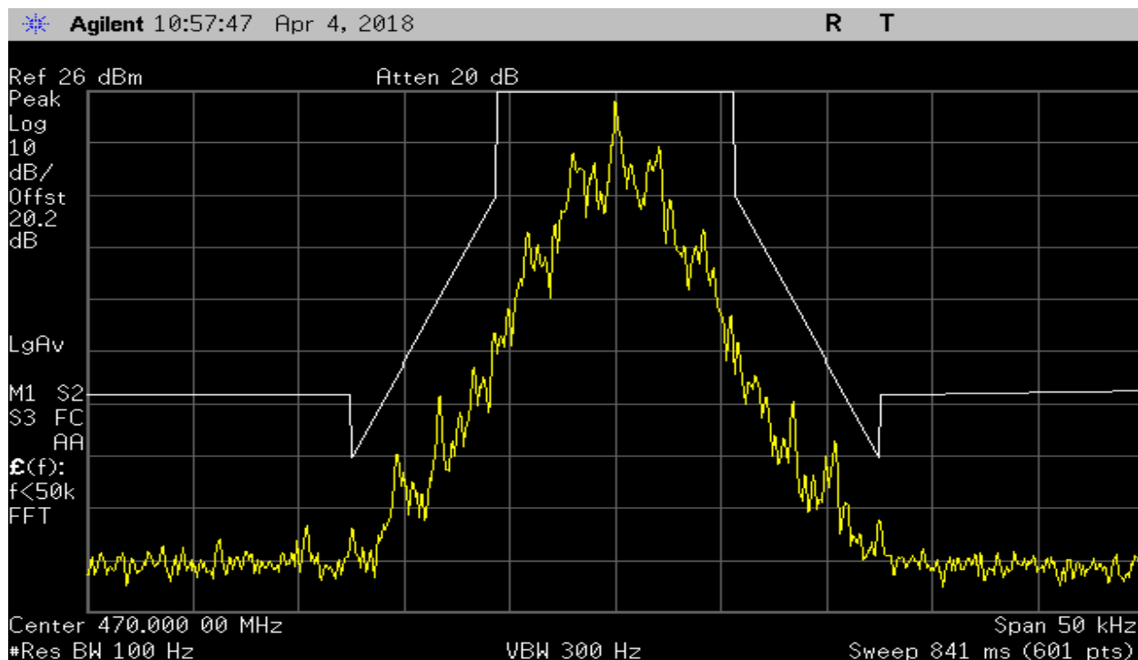
Plot 6 – Mid Chanel 12.5 kHz Spacing – Mask D
