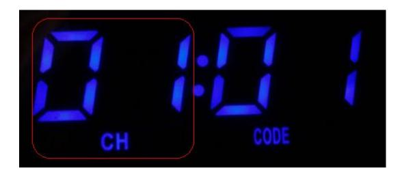
**CODE Code:** 00--99 Code: through code code can reduce external interference, please note that CODE code and communication channel set the same channel to establish talkback.
