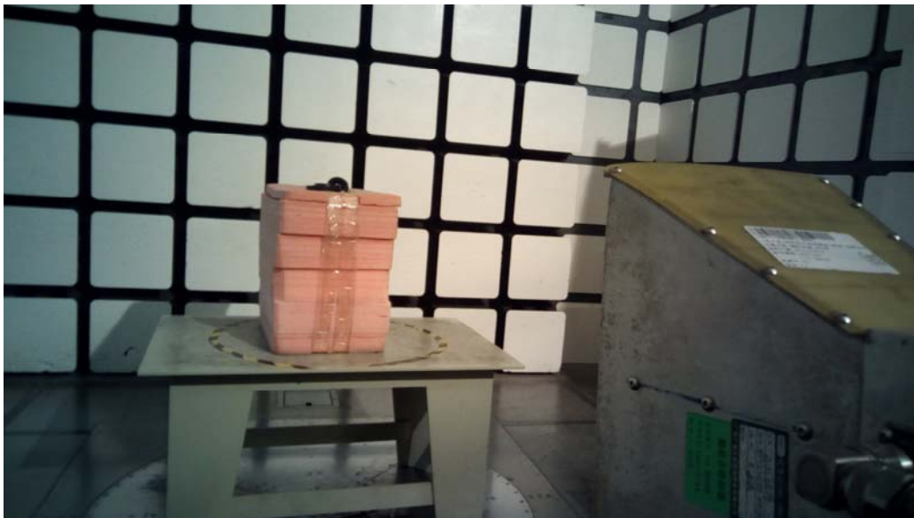
Radiated Emissions View (Above 1 GHz)
