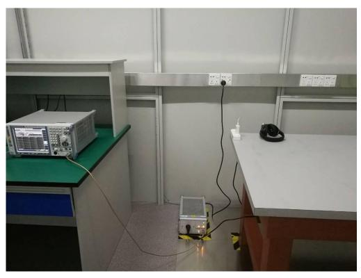
FCC RADIATED EMISSION TEST SETUP
