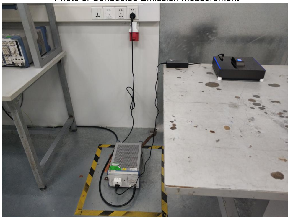
FCC ID: 2AQQO-1080 Photo of Conducted Emission Measurement
