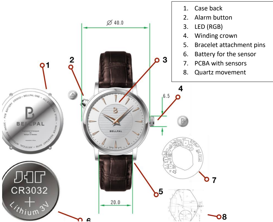
Figure 1. The parts of the watch
