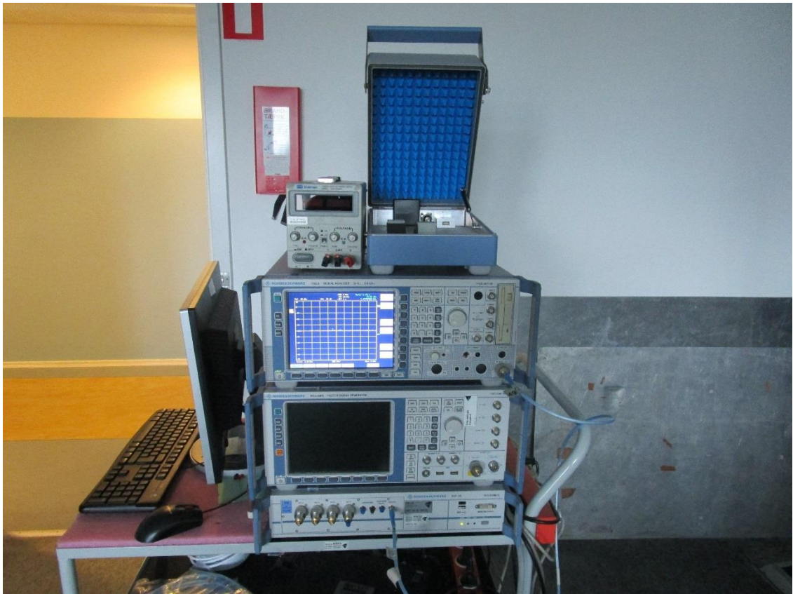
Photo 4.9.1 Test setup regarding measurement of 20 dB bandwidth.
