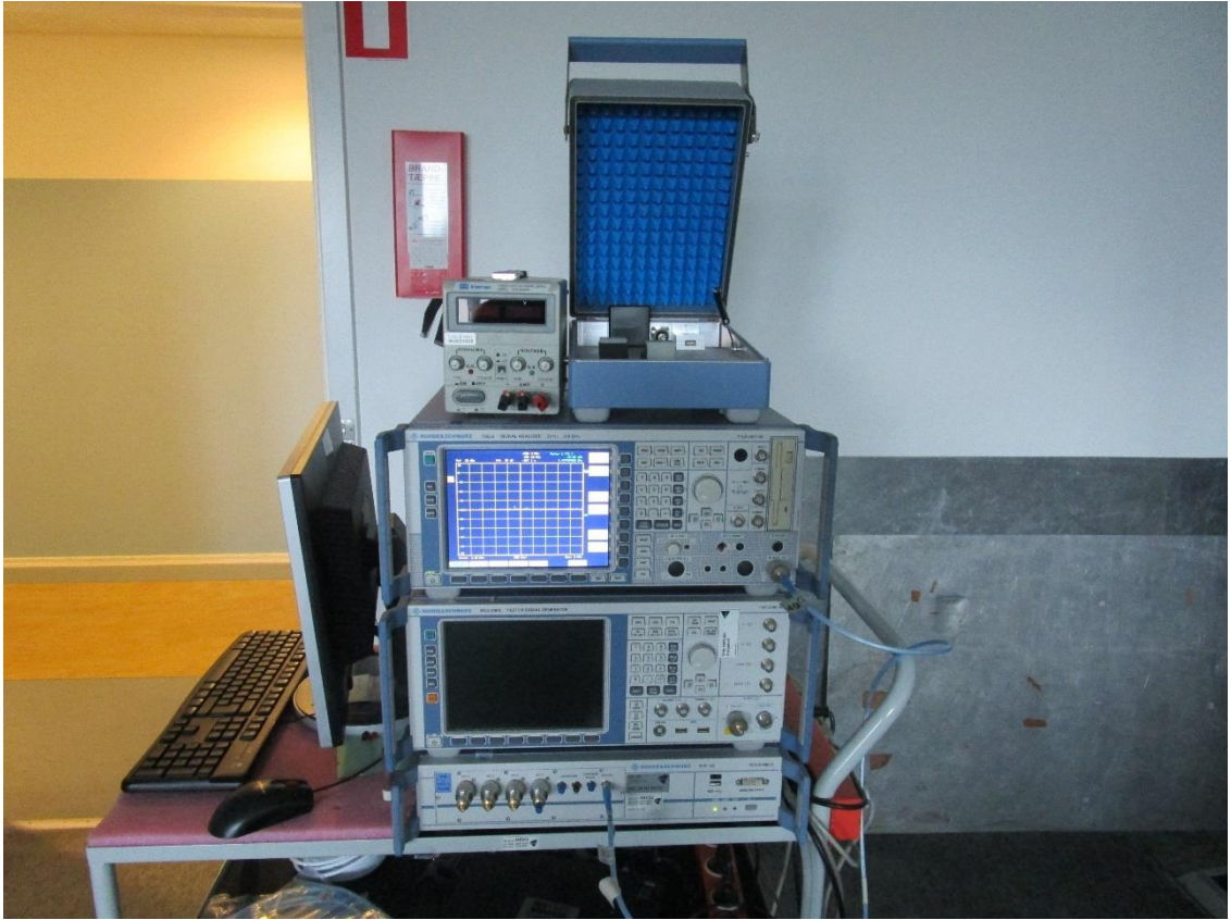
Photo Error! No text of specified style in document..7 Test setup regarding measurement of 20 dB bandwidth
