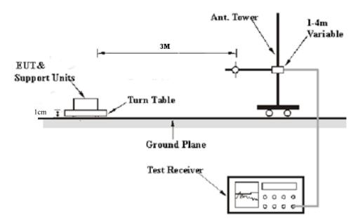
The radiated emission tests were performed in the 3-meter chamber a test site, using the setup accordance with the ANSI C63.10. The specification used was the FCC Part Subpart C limits.
