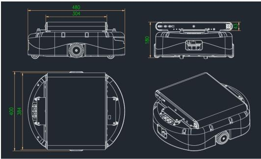
Rated Load: 20kg Transfer way: Belt Drive drive system: Servo Motor Set speed: 1.5m/S Set acceleration: 1.5m/S<sup>2</sup> Communication mode: Wireless Working temperature:-10 ~ 55° Humidity: ≤95% (25°C) RH LIB: 4.6VLi-Ion 92Wh Charging voltage: 4.6-5.4V MAX Charging current: 90A Endurance: 3H
